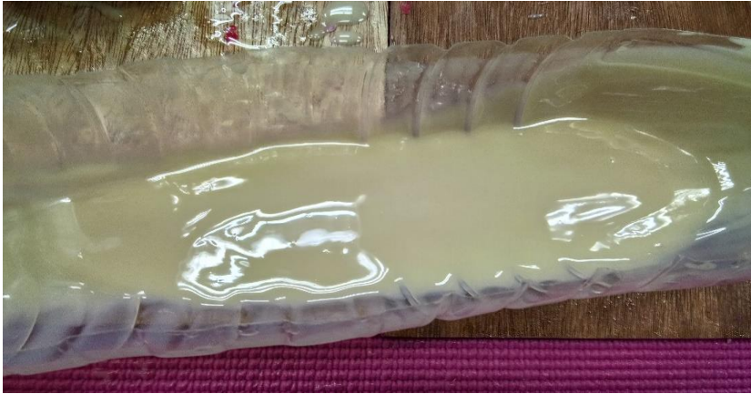
Figure 2.10 Disclosed PU (Part A) solution after mixing with the hardener (Part B)
