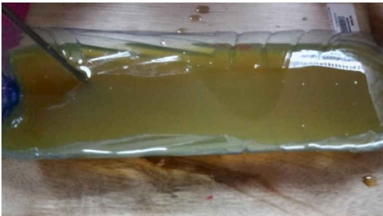
Figure 2.9: Portrayed PU (Part A) solution before mixing with the hardener (Part B)
