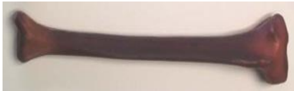
Figure 2.2 Depicts fourth generation of large tibia composite model from Sawbones(2)
