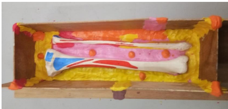
Figure 2.8: Depicted the placement of tibia and fibula adhered by plastiline.
