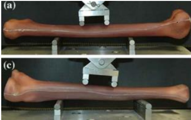
Figure 2.4 Specifies four-point bending test setup of the fourth generation of Sawbones ' large tibia composite model (2)
