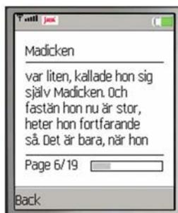
Figure 8 Paging implemented on a mobile phone
