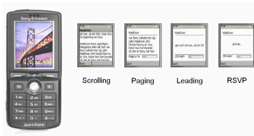
Figure 23 The Sony Ericsson K750i mobile phone used in study four (left) and the presentation formats in the same scale (right), see figure 4-7 for close-ups
