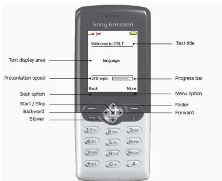
Figure 11 Button assignments for RSVP on a Sony Ericsson T610 mobile phone
