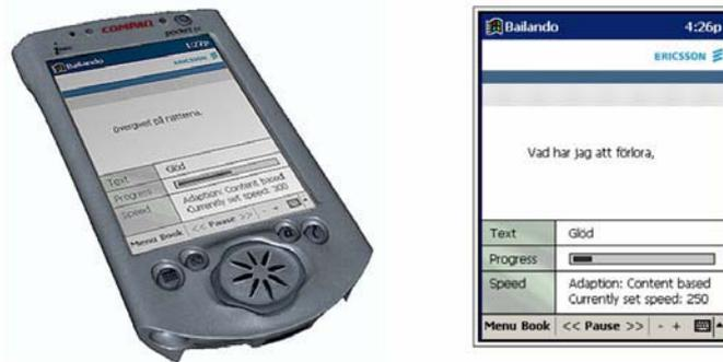
Figure 12 The Bailando prototype on a Compaq iPAQ 3630 (left), view of the RSVP interface (right)
