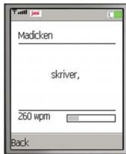
Figure 10 RSVP implemented on a mobile phone
