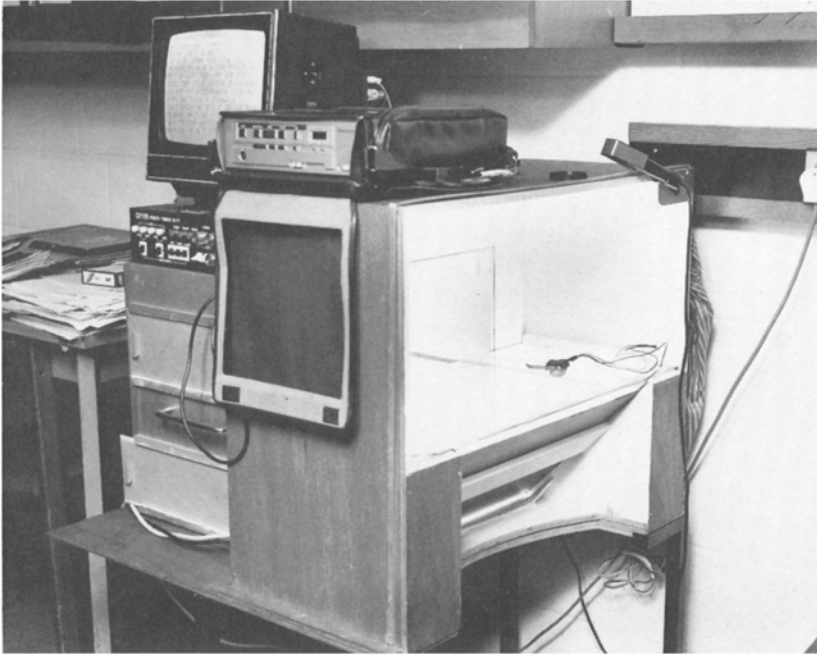
Figure 3.1 Photograph of the recording apparatus, seen from the subject's side. The experimenter sits on the left, facing the monitor, videotimer and recorder, and the shutters through which the camera and lens can be adjusted if necessary
